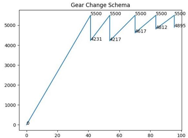
The optimal engine speeds in gear for the redesign gearbox:
