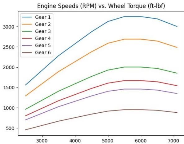
While these graphs are useful in visualizing the array of data for each gearbox, they lack necessary insight into how to make performance-based design decisions. Specifically, these graphs do not provide enough information on how gear changes should be executed to drive the race car at near-peak capabilities. For this reason, the existing data was refactored into the following graphs that show land speed versus torque. For the baseline gearbox that looks like:
